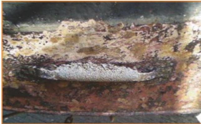
*Anode loss & hull damage accelerated by shore power connection. The vessel next to this narrow boat failed to fit anode protection but **neither** boat was isolated: This allowed the adjacent vessel to use the anodes on this boat & resulted not only in the severe corrosion illustrated but two very unhappy sailors! This type of corrosion is easily prevented by fitting a galvanic Isolator. This also prevents your neighbour "borrowing" your anodes.*
