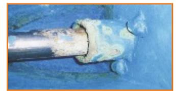
*The **four** pictures above were taken from a princess GRP cruiser which was surveyed 2005 & was in perfect condition. Eight weeks later after connection to a defective shore power outlet this was the result! The brass inlet grill was eaten away, skin fittings almost dissolved, stainless steel shaft pitted & just look at the props! The repair bill was £6000! An isolator with status monitor would have prevented this!*
